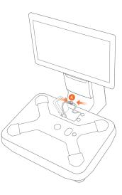
4 Connect the scale body with the main screen and then close the rubber cover.
